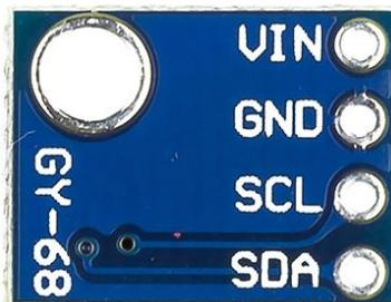
In your kit, both this BMP180 and the OLED screen use I2C and each have unique addresses. You may notice that the OLED allows for device address changes by moving a small SMD resistor on the back side of it's board.
